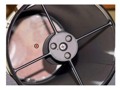
Most telescope constructions adjust the secondary mirror by three loaded screws like those (allen head screws) shown here in the picture.
