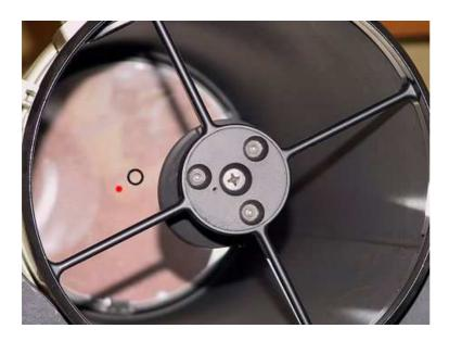
Picture 1 left shows the laser beam (red dot) obviously missing the marker circle in the center of the main mirror. Note the three adjustment Hex head screws of the secondary mirror spread 120° apart. Very cautiously and only in small steps re-tilt the secondary mirror by very slowly tightening and releasing these adjustment screws.
