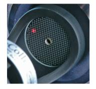
If you see this on your reference plane, adjust (tilt) your main mirror in a way that the laser point passes exactly through the center hole thus being reflected into itself.
