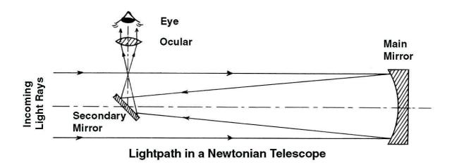
**The incoming light** travels first from left to right to the main mirror at the end of the tube, is reflected there and travels right to left, to the secondary mirror, which in turn deflects the light out of the tube and – via the eyepiece – into your eye.
