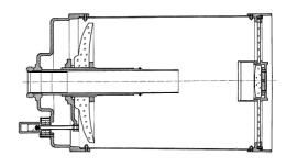
Simplified sketch of the SC-secondary mirror tilting mechanism. Three screws are arranged 120° apart, around a center pin on which the secondary mirror pivots. Loosening one screw and tightening another will tilt the mirror into the designed position.
