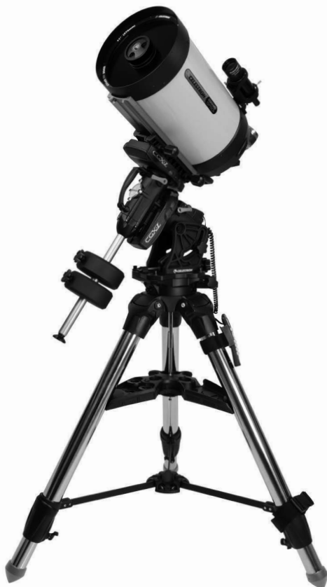
Figure 7 Telescope in the home position
