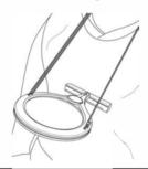
2. To turn LED light ON/OFF, slide switch up/down
