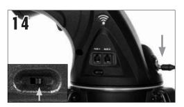
Verify that the small Wi-Fi switch above the power switch is in the right position. Then, turn on the power switch at the base of the motorized fork.
