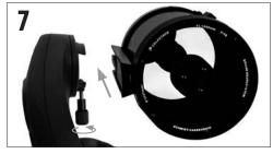
Attach the telescope optical tube by positioning the dovetail into the dovetail holder on the fork arm. Make sure the bottom of the dovetail is flat against the dovetail holder. Firmly tighten the thumb bolt.
