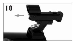
Slide the finderscope bracket into the dovetail slot on the telescope tube near the focuser. The large window on the finderscope should be facing the front of the telescope. Secure the bracket by tightening the setscrew on the dovetail slot.
