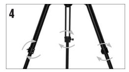
Extend the legs of the tripod by loosening the three hand knobs on each leg. Pull each leg section all the way out and tighten the hand knobs down to secure them in place.
