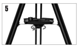
Thread the captive hand bolt in the center leg brace through the bottom of the accessory tray to secure it in place.
