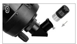
Insert the barrel of the 25mm eyepiece into the top of the star diagonal. Tighten the setscrew.
