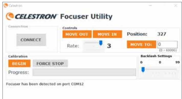
The free Celestron Focus Utility Program provides a simple user interface for controlling the focus motor.
