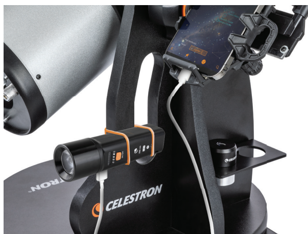
Figure 13a: The PowerTank Glow 5000 mounts to the cutout handle in the base using the bands which come with the PowerTank.
