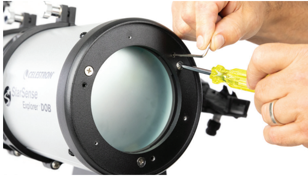
Figure 20: For the 130 Tabletop Dob, three sets of push-pull screws in the mirror cell adjust the primary mirror's tilt. Loosen one screw in the pair and tighten the other to adjust the tilt.
