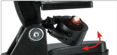
Illuminate the slide by using the mirror to reflect light from a lamp or other light source into the microscope or by rotating the light bulb assembly upwards until it turns on. Aim the light source by tilting the mirror/light assembly until the view in the eyepiece is evenly lit.
