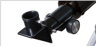
Loosen the set screw on the back of the focusing assembly and insert the star diagonal. Secure the diagonal in place by tightening the set screw on the focus assembly.
