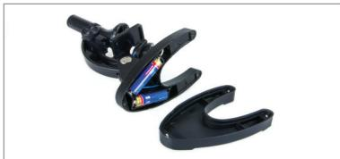
Your microscope comes completely assembled but you will need to insert two AA batteries in order to use the built-in illuminator. Start by removing the three Phillips head screws under the bottom plate. Pull the plate off the base of the microscope. Insert batteries into the battery holder making sure to insert them in the correct polarity. Replace the base plate and screws.
