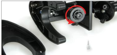
Your microscope comes with a spare light bulb for your illuminator. To change the bulb, remove the batteries and turn the illuminator so you can access the light bulb. Turn the ring around the light bulb 1/8th of a turn counterclockwise to unlock the ring. Lift the ring upward to expose the bulb. Replace the bulb and replace the ring by pushing it toward the body of the illuminator and turning it clockwise to lock it in place.
