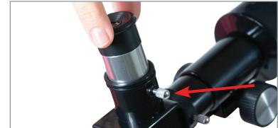
Loosen the set screw on the star diagonal and insert 10mm (60x) eyepiece. Secure the eyepiece in place by tightening the set screw on the star diagonal.
