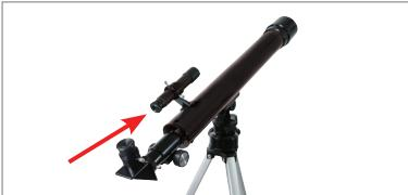
Point the telescope at a distant target by sighting through the finderscope.
