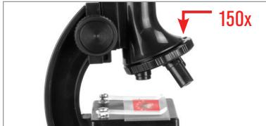
Rotate the objective lens turret until 150x appears in the magnification window. The turret will click into place when it is aligned correctly.
