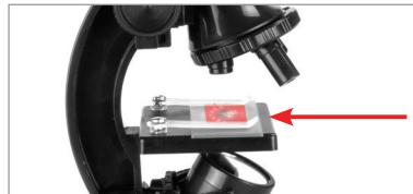
Insert a prepared slide into the clips on the microscope stage.
