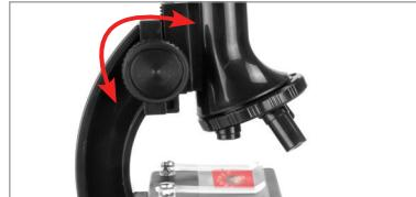
Look through the eyepiece and turn the focusing knob slowly to lower the objective lens toward the slide until you can achieve a sharp focus. Be careful not to move the microscope down too far so that the objective lens makes contact with the slide or damage to the slide or microscope may occur.
