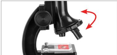
To increase magnification, turn the focuser so that the eyepiece is raised to its fullest height, then rotate the turret until 450x is shown in the magnification window. Focus again by moving the microscope downward slowly until focus is achieved. Repeat this procedure for 900x.
