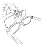
2. Place clamp around bridge of glasses frame and release clamp when in place.
