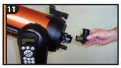
Insert silver barrel of diagonal into the visual back as shown above. Tighten silver screw to secure.
