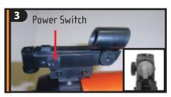
Now you will need to align the finderscope. Turn on the red LED light by turning the knob shown above. When used for the first time, remove the clear plastic disk that is located between the battery clip and the battery. See inset.
