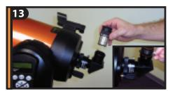
Insert silver barrel of 25mm eyepiece into the diagonal as shown above. Tighten silver screw (inset) to secure.
