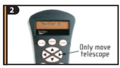
You will notice that there are directional arrows in the center of the hand control. These **only** move the telescope. **They cannot be used to scroll through menu features.**
