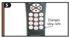
In order to accurately center an object in the eyepiece it may be necessary to change the slew speed of the motors. To change the slew speed, press the RATE button then select a number from 1 (slowest) to 9 (fastest).
