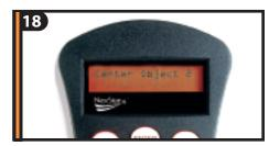
For the second alignment object, choose a bright star or planet as far from the first alignment object as possible. Once again use the directional arrow buttons to center the object in the finderscope and press ENTER. Once object is centered in the eyepiece, press ALIGN.
