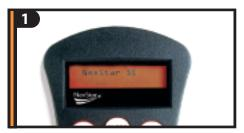
Turn power switch (located at the base of the fork arm) to "on" position. The light will come on and the hand control will display "NexStar SE".
