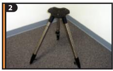
Assemble tripod by spreading the legs out until fully extended.
