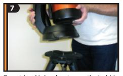
Once tripod is level, put away the bubble level. Grab scope by the fork arm and line up holes on bottom of telescope with the screws on the tripod mounting platform.
