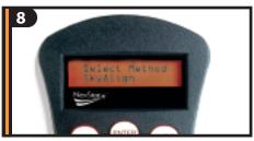
When the display reads NexStar SE, press ENTER to begin the alignment procedure.
