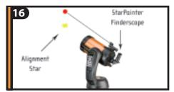
If the finderscope has been properly aligned, the alignment star should now be visible in the field of view of the eyepiece.
