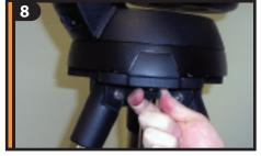
Tighten three screws under tripod mounting platform to secure the fork arm to the tripod.
