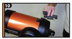
Slide StarPointer finderscope onto mounting platform as shown above. Tighten screws located on side of StarPointer to secure.
