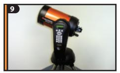
Hand control comes mounted in the fork arm. Hand control should fit snugly in fork arm as shown above.
