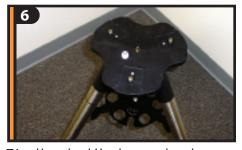
Tripod legs should be the same length to provide a level platform for the telescope. A bubble level is included to assist in leveling.
