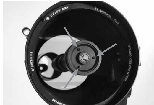
Secondary Mirror Collimation Adjustment Screws
