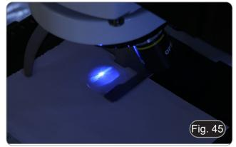
6. Using the centering screws ③ on the side of the lamp housing, center the image of the arc. (Fig. 45-46)
