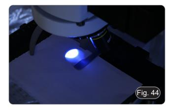
5. Using the focus screw of the collector lens ②, put the image of the arc projected onto the paper. The light spot must be brighter and sharper as possible. (Fig. 45)
