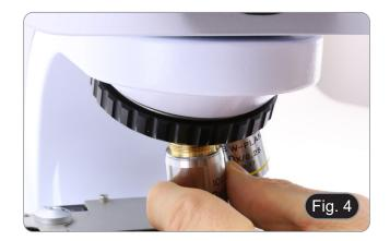
4. Screw each objective into the thread of the nosepiece, clockwise with increasing magnification. (Fig. 4)
