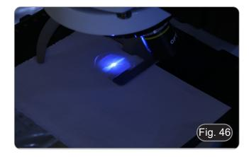
Using the focusing screw of the collector lens 2 enlarge the image until a homogeneous illumination is achieved (Fig. 47). At this point, insert an objective into the optical path and, looking into the eyepieces, optimize the illumination always using the screws 2 and 3.
