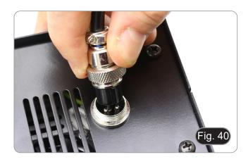
5. Insert the power cord into the connector (5). (Fig. 41)
