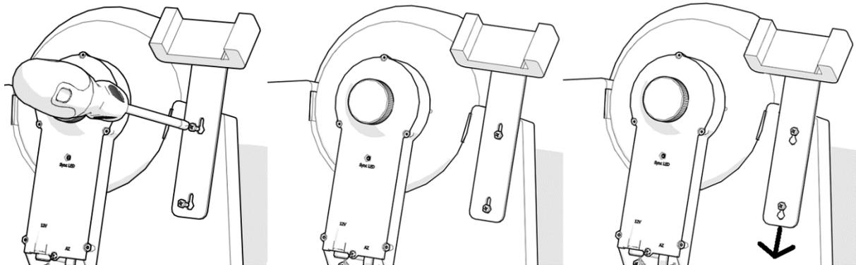
**3.1. Adjusting the position of the smartphone.** Adjust the smartphone's position if necessary (vertical or horizontal position) and fix it using the supplied hex screw (part #11) as shown.
