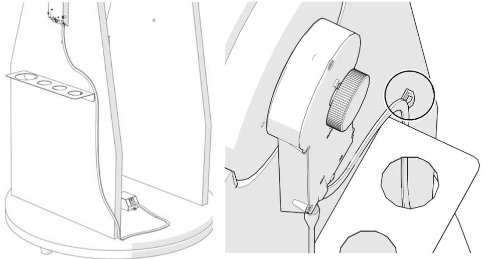
**3. Installing the Smartphone Holder.** The smartphone is an important part of the setup and a smartphone holder was included. Use the smartphone holder (part #9) and fix it with the two supplied screws (part #10) using a screw driver (not included). Apply some pressure to the screws so they pierce through the wood. Note that the screws should not squeeze the metal but allow it to slide if necessary. Remove it whenever required (transportation).
