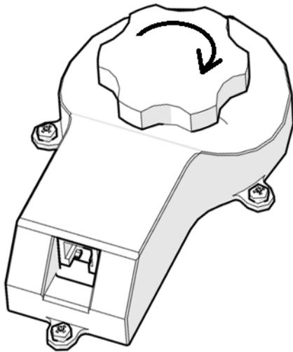
Insert the original hand knob, supplied with the telescope, through the hole and tighten it firmly.
