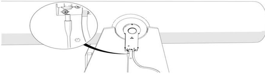
Then plug-in the power cable jack to the Altitude Encoder and Bluetooth® Box. The Red LED will start blinking.
