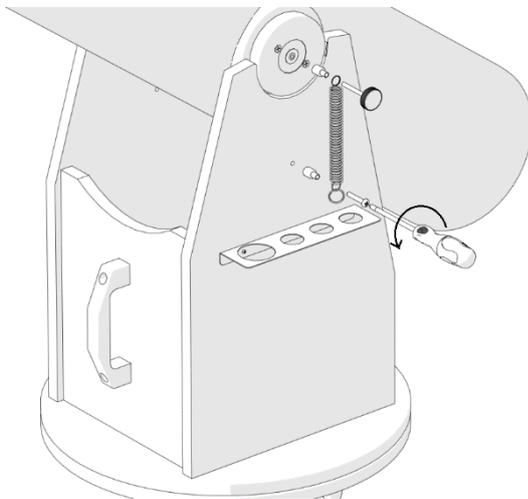
**2.3. Installing the Altitude Encoder and Bluetooth® Box.** Now that you have fixed the Azimuth Encoder, install the Altitude Encoder and Bluetooth® Box to the base.
