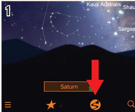
**1.** First, tap the StarSense icon. The app will ask you if your telescope is aligned. If you removed your phone from the Dock since the last time you aligned, it's probably a good idea to complete the process again. Press Needs Alignment to begin. It will only take a minute.
