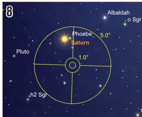
**8.** If the telescope has detected stars, but is still not over your intended target, the bullseye will turn yellow. Continue to follow the arrows closer to the target.
