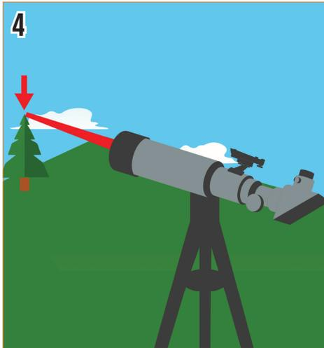
4. Next, we need to align the phone's view to the telescope's view. To do this, start by pointing your telescope at a very distant object. It's best to choose an object that's at least a quarter-mile away.
